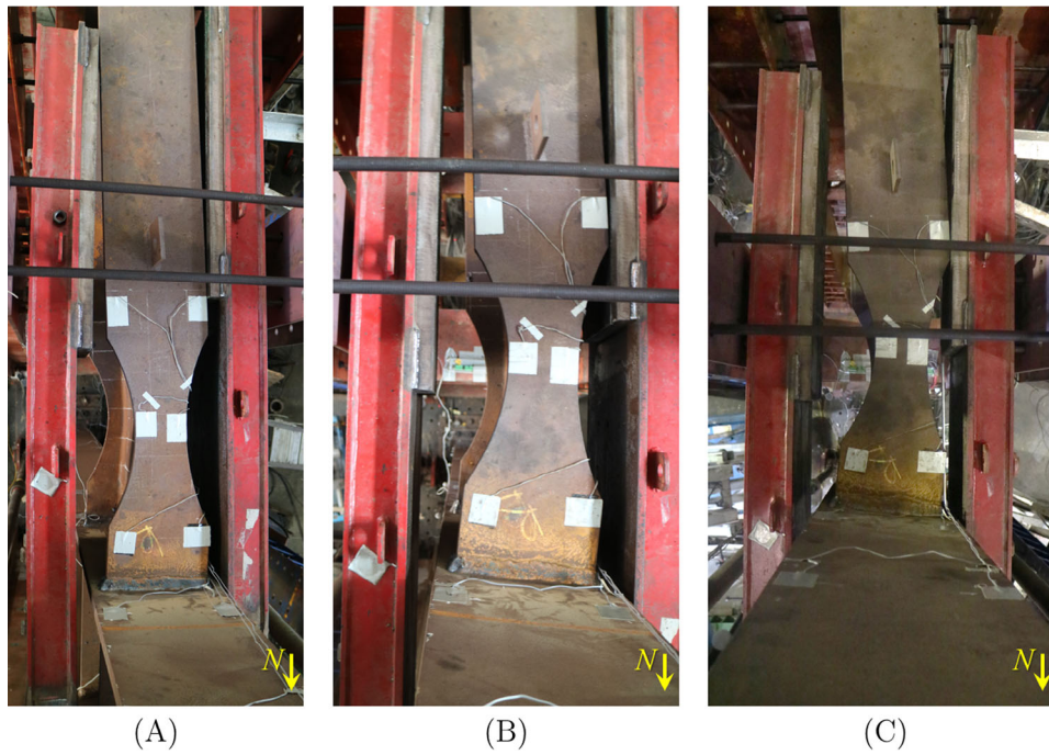
FIGURE 20 | Sequence in beam lateral buckling: (A) HS-A2; (B) HS-A3; and (C) HS-A4.
