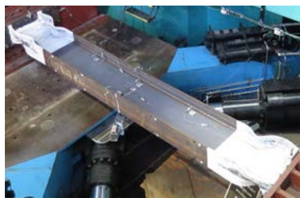
(b) Anti-symmetric local buckling
