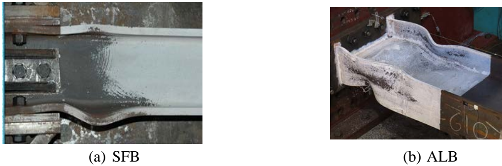
Fig. 2 Symmetric flange buckling and antisymmetric local buckling
