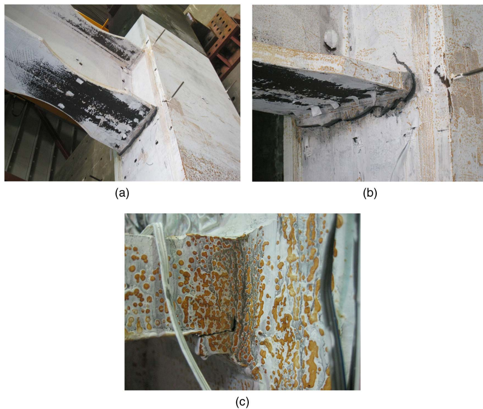
Fig. 6. Specimen 2: (a and b) fracture at beam bottom flange level at +3.9% drift; and (c) fracture at beam top flange level at -3% drift (second cycle).
